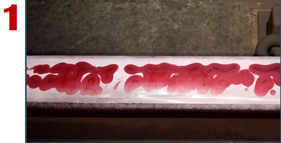
Dye penetrant testing is used to clearly identify defects
